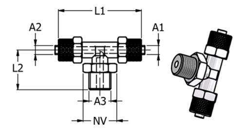
Hose diameter A1 = 6/4Hose diameter A1 = -Hose diameter A2 = 6/4L1 = 39L2 = 26.0NV = 16Thread A3 = G 1/4"
